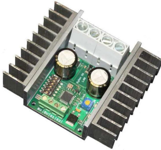
Figure 38: Syren 50A Motor Controller
