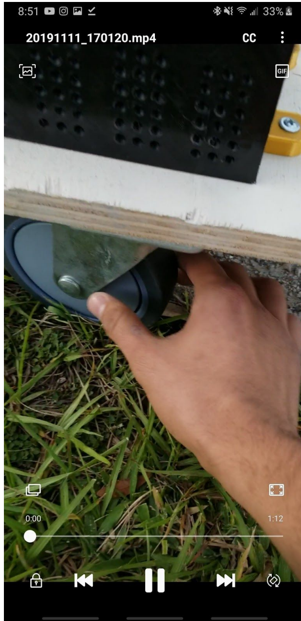
Figure 71: alphagoat getting stuck because swivel wheel
