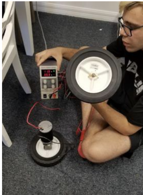
Figure 68: Power supply testing that old wheel motors work correctly
